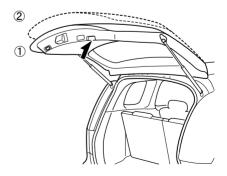
If the vehicle battery is dead or there is a malfunction in the electrical system and the liftgate cannot be unlocked, perform the following procedure as an emergency measure to unlock it:
